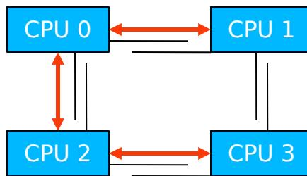
Need to propagate write on Bus 2-3 (or 1 – 3)
